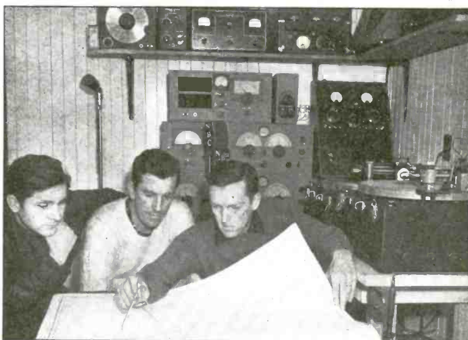
2—The Fahnestock boys, charting their course on a map of the South Pacific ocean. The radio equipment (a philanthropy of Helen Fahnestock Hubbard) aboard their 137-ft. long 3-mastered schooner, Director II , includes the following: transmitters , 1—1,000-W., on 3 to 30 mc. (listen for KWAH); 2—100-W., for expeditionary use, on 6 to 30 mc. and 7 to 60 mc.; a 20-W. ultra-H.F. launch portable on 40 to 112 mc.; 2—3-W. ultra-H.F. 7-lb. pack units on 40 to 80 mc.; 2—1/10-W. portables on 112 mc.; 1—60-W., 600-meter emergency unit; and, a 5-W., 3 mc. airplane unit. Receivers cover 90 to 112 kc.
